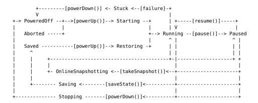
Note that states to the right from PoweredOff, Aborted and Saved in the above diagram are called *online VM states*. These states represent the virtual machine which is being executed in a dedicated process (usually with a GUI window attached to it where you can see the activity of the virtual machine and interact with it). There are two special pseudo-states, FirstOnline and LastOnline, that can be used in relational expressions to detect if the given machine state is online or not:
