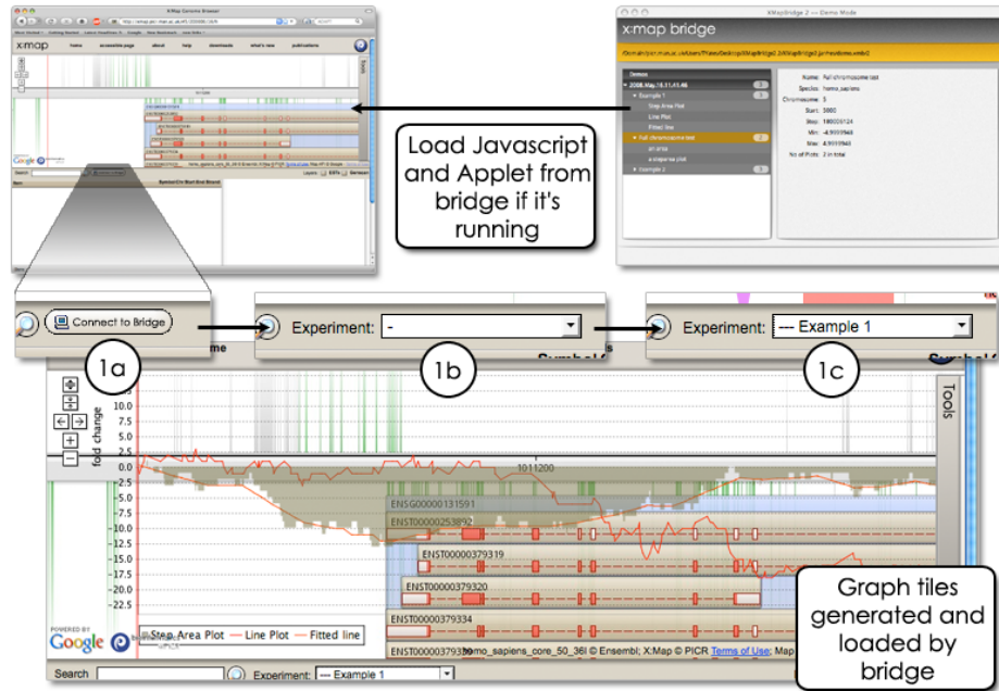
Figure 2: The process to show the graphs in the browser (1a) Click on the connect button (1b) This changes into a drop-down select box (1c) select the graph of choice
