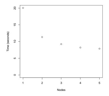
Figure 1: Execution time decreases asymptotically with number of nodes. The decreasing performance gain is primarily due to communication overhead.
